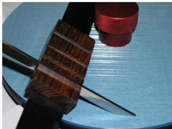
Narrow Chisel held in Saddle on Tool Bar
